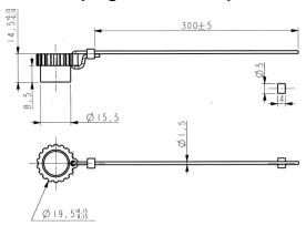
◆ Elastomer cap with crimped eyelet diameter 3 for JDX T2 receptacle
