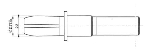
Connector without locking equipped with 7 flat cts
